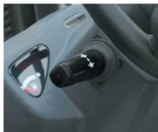
Finger-tip operation with the electric F/R lever
