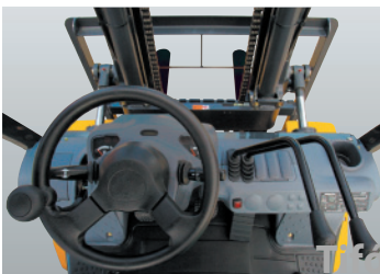
Finger-tip operation with the electric F/R lever
