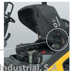
Locking engine hood provides protection while servicing
